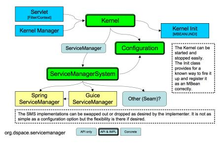
The DS2 kernel is compact so it can be completely started up in a unit test (technically integration test) environment. (This is how we test the kernel and core services currently). This allows developers to execute code against a fully functional kernel while developing and then deploy their code with high confidence.
