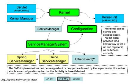
The DS2 kernel is compact so it can be completely started up in a unit test (technically integration test) environment (this is who we test the kernel and core services currently). This allows developers to execute code against a fully functional kernel while developing and then deploy their code with high confidence.
