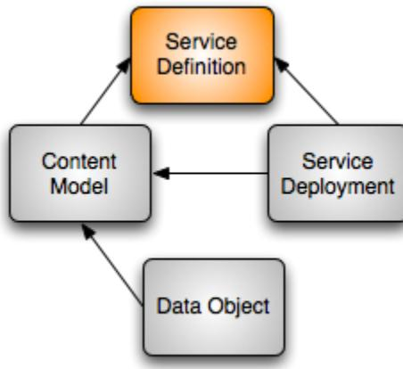
This guide describes how *Service Definition Objects* are constructed in detail. In Fedora, a Service Definition ("SDef") is a special kind of object that defines a set of operations on objects in a repository. As you will see, that set of operations needs to be expressed in a particular way inside the object in order for Fedora to understand it.
