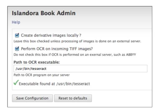
If you wish to use external services for image derivation and OCR, deselect these boxes. You will need to make sure that the path to your version of tesseract (that has been installed in the same server) is identified in "Path to OCR executable." A green check mark will appear to indicate that the system has discovered the tesseract directory.
