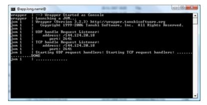
2) Shutdown the handle server by executing CTRL^C in the command window and select Y.
