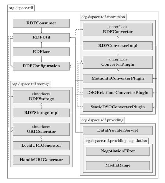
The classes RDFConsumer and RDFUtil integrate dspace-rdf into DSpace. RDFConfiguration is used to centralize configuration properties used by more than one class inside dspace-rdf. The class RDFizer contains the command line interface. To see the online help you have to use the following command:
